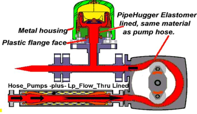
Best of all, because of large diameter it takes part of a psi only for diaphragm response. In-line flush through.
