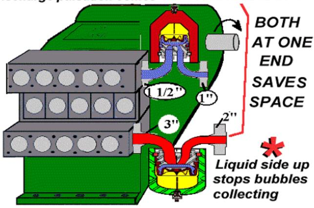
No flow reversals in a single connection, 300% better suction performance. Saves using 3" suction line. Down sized to 2", saved more than cost of Pipehugger LP suction dampener.
