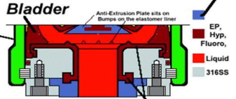
Replaceable elastômer liner in same material as liquid bladder
